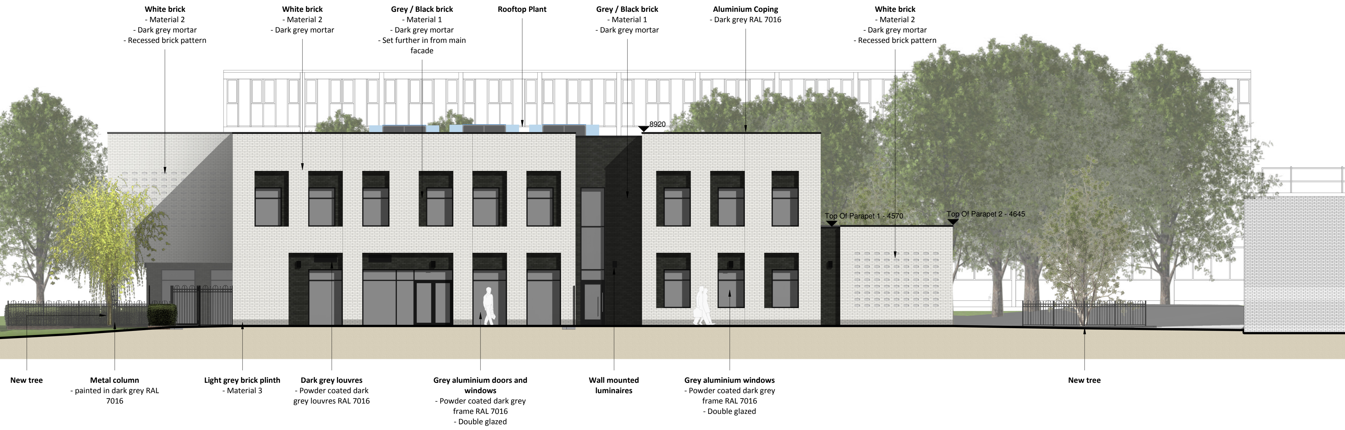
2 Elevation 2 - East Elevation 1 : 100
